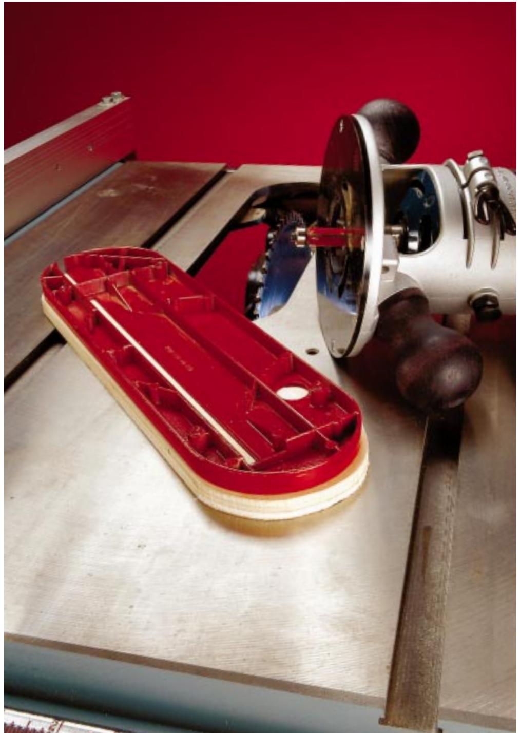
Photo shows the insert blank after being bandsawn to rough shape, but prior to being routed to exact shape.
